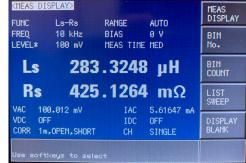
**7** Once the DC bias level is increased above the saturation point of the core, the inductance of the transformer drops. see below, **102.2uH** @ **3A DC**
