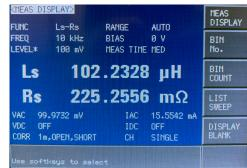
By taking several readings over the range, you can easily plot a graph to show the characteristic saturation curve of the UUT.
