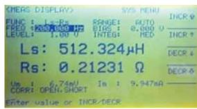
By taking several readings over the range, you can easily plot a graph to show the characteristic saturation curve of the UUT.
