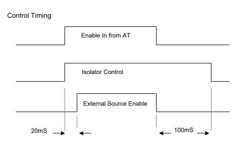
The diagram above shows the signal levels (high or low) and the times between them from when the AT3600/AT5600 asserts its enable signal. The Enable In (from AT) is not visible on any ACIF ports. It is a control line that comes in from the AT3600/AT5600 peripheral port.
