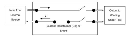
Test current flows from the external source into the fixture and out to the winding under test via an isolation relay. The current returns through the fixture via another relay and a current sensing transformer or shunt that must be fitted to the interface. A standard 1:20 current transformer is supplied with each interface.
